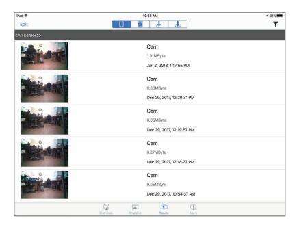
**Note:** When locating recordings using an iOS device, you'll see four icons at the top of the screen that point you to recordings: on the mobile device, on the microSD card, downloaded from the camera to the mobile device or currently being downloaded.
