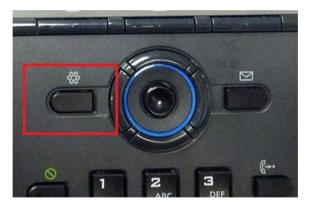
2. Scroll through the Configuration Menu and select Lock/Unlock Config.
