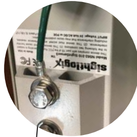
Camera must be grounded via mounting bolt to earth ground rod (or equivalent)
