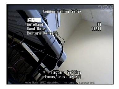
The Bosch PTZ Setup menu options should be configured as shown.
