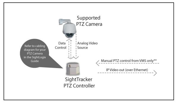
\*\*Note - Manual control of the PTZ over Ethernet is possible via your VMS joystick and/or keybord. Do not connect a keyboard directly to the SightTracker to manually control a PTZ.
