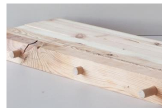
Figure 13. Small scale ceiling sample with dowels
