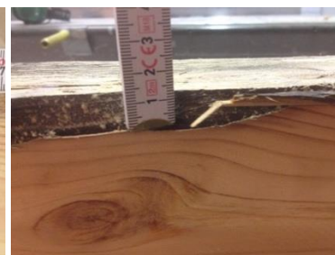
Figure 5. Strength grading: assessment of lamellas regarding dimension, location and orientation of branches, defects, decays and cracks.
