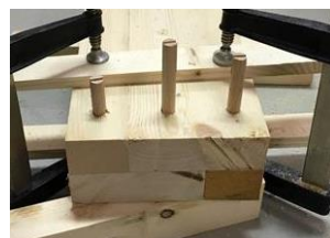
Figure 11. Dowels for fixation of lamellas
