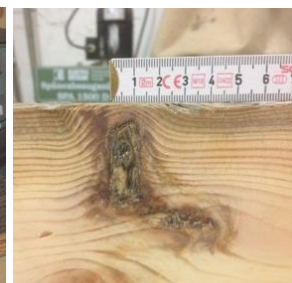
Figure 5. Strength grading: assessment of lamellas regarding dimension, location and orientation of branches, defects, decays and cracks.
