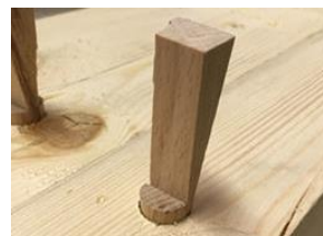
Figure 12. Wedges for fixation of dowels
