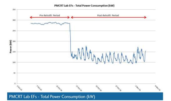
Aircuity's exhaust fan application was implemented. UHN then extrapolated those savings to get annual savings of 1,550,000 kWh (equivalent to 160 houses in Ontario) and electric peak demand savings of 111.7 kW (equivalent to running 1,400 flat screen TVs simultaneously). This equals a cost savings of \$200,000 annually. When coupled with savings from the previous Aircuity lab project in PMCRT, the reduction in utility costs through Aircuity equals approximately \$1,000,000 annually.
