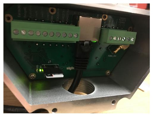
Note that the yellow light to the left of the green indicator light will flash when the card is actively recording (after it has been formatted, described below).
