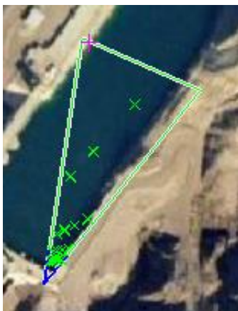
A scattered distribution can indicate a poor calibration.
