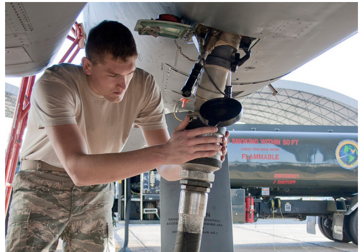
US Air Force, Public Domain | Senior Airman Jacob Prine checks the fuel connection prior to a flight test of new, environmentally-friendly fuel.
