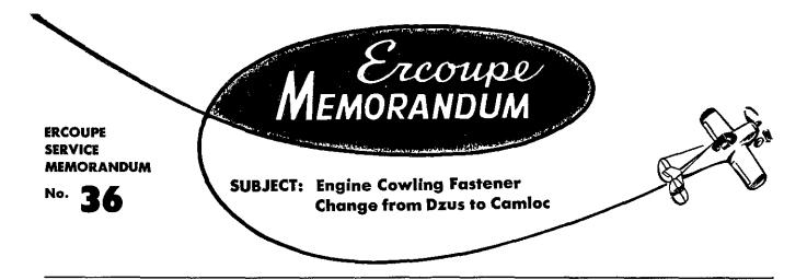
1. Effective on all Ercoupes serially numbered 2623 and subsequent, the engine cowling will be secured with Camloc fastener. It is believed that the use of Camloc fasteners will provide a better cowling fit and simplify maintenance due to superior design. This type fastener will also provide easier access to the engine.
