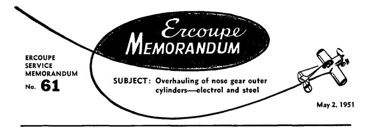
Service experience in the past two years has indicated that it would be desirable to provide certain service parts to improve the life of the Outer Cylinder for the steel nose gear, part #415-34080. We also found the need for oversize pins to permit the salvaging of the Outer Cylinder in the Electrol strut, part #415-34324 and its associated parts. We have, therefore, developed and obtained approval on the following rework on these items.
