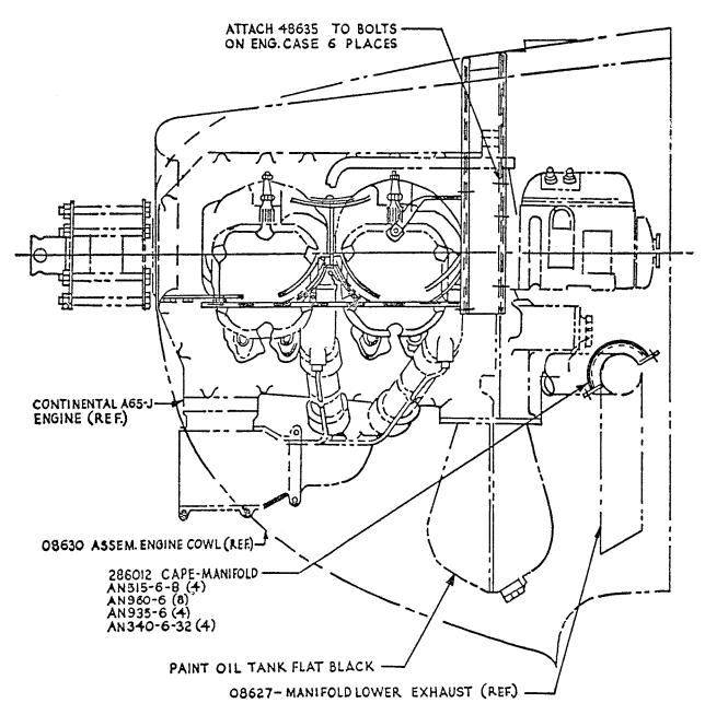
NOTE: THIS IS A PRESSURE BAFFLE SYSTEM BAFFLES MUST FIT TIGHT ON ASSEMBLY.
