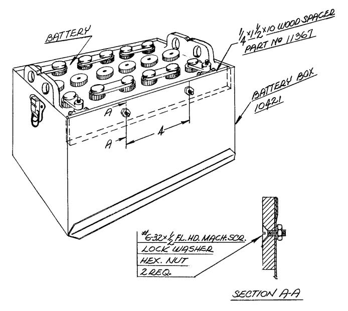
BATTERY SPACER INSTALLATION
