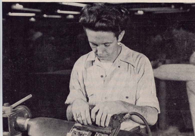
6—(Above) With the blade covered with the plastic sheet, it is left to cure after which overlap is cemented flat on the thrust face. 7—(Below) Sanding of the cured blade is accomplished after the lap joint has been cut off. Templates are used to check uniformity
