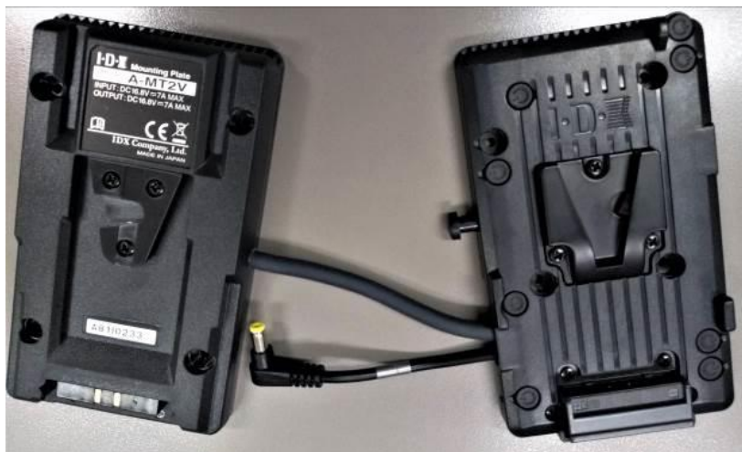
Photograph 9, 10, 11, 12 ,13 Mounting Plates assemblies options - LU300S-VM-5G
