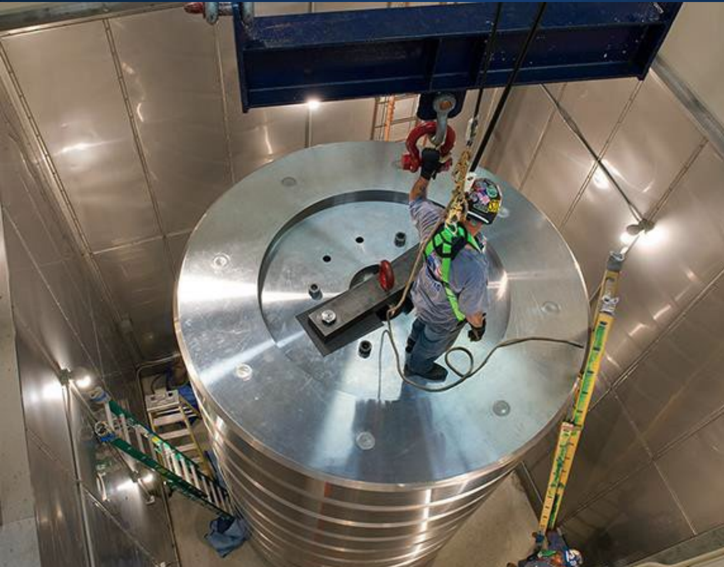
Million Pound-Force Deadweight Machine for calibrating force sensors
