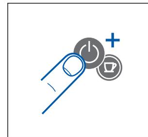
12. Exit: press both buttons simultaneously for 3 secs
