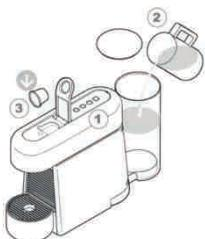
**① Turn the machine on** and wait for it to be in ready mode (steady lights). Fill the water tank with fresh potable water and insert the capsule.
