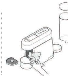
**② Dry with a fresh and clean towel**, cloth or paper and reassemble all parts. Clean the coffee outlet and inside the machine regularly with a damp cloth.
