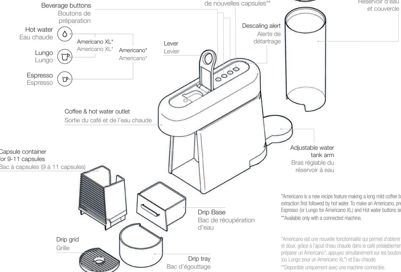
\*Americano is a new recipe feature making a long mild coffee based on coffee extraction first followed by hot water. To make an Americano, press both the Espresso (or Lungo for Americano XL) and Hot water buttons simultaneously.
