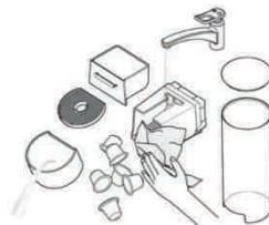
**① Empty the drip tray**, the drip base and the capsule container every day. Also remove the water tank with its lid and clean them all with odorless detergent and rinse with warm / hot water.
