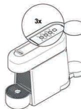
**② LEDs will blink** fast 3 times to confirm machine has been reset to factory settings. Machine will then switch off automatically.
