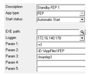
In standby mode, the FEP will not run any receiver drivers, but will instead run a single standby poll thread. This thread will connect to the primary FEP's standby delivery thread to receive signal packets. Note, while in standby mode, the FEP does not start a control listen thread, so the FEP Commander will not connect.
