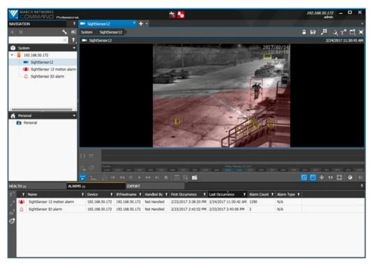
The motion alarm should be logged in the March Command Management [CRI console].
