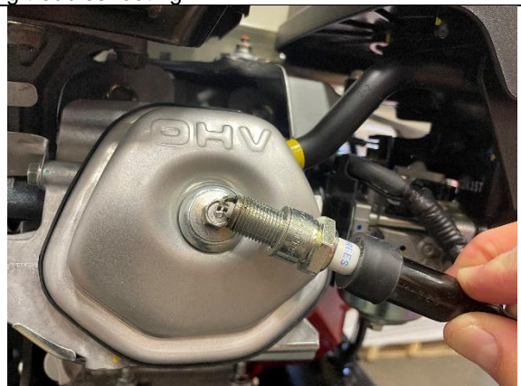
Spark plug grounded against valve cover bolt
