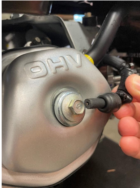
Spark plug lead against the valve cover bolt.
