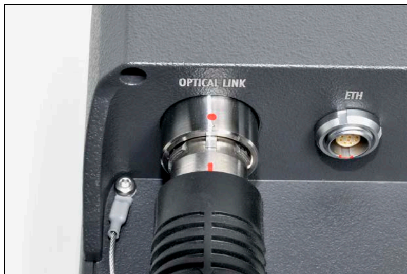
Figure 133: Correctly aligned fibre connectors
