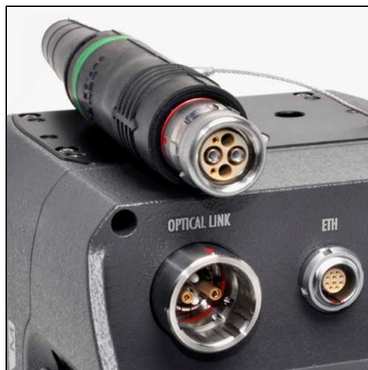
Figure 132: SMPTE 311 optical fibre connectors
