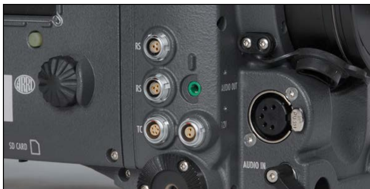
Figure 16: 24 V outputs (RS) and 12 V output
