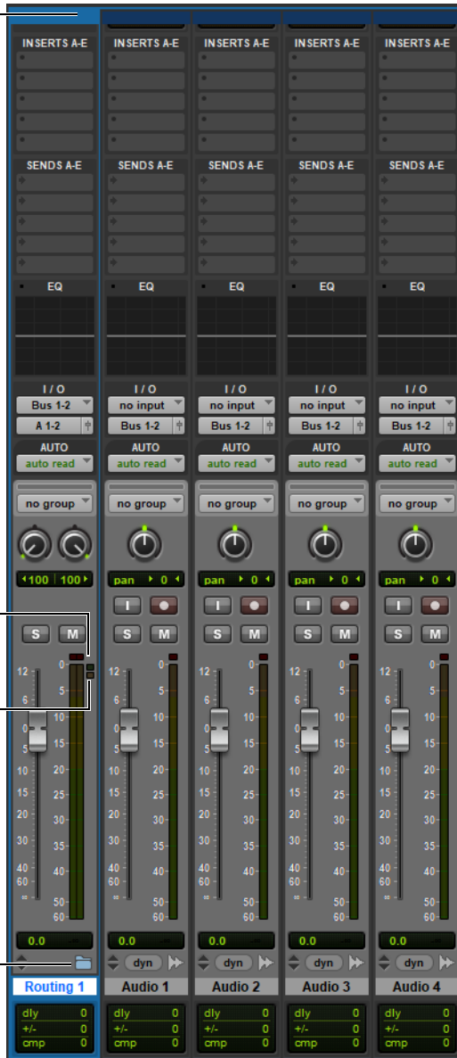
Mix window, Routing Folder track open—output of contained audio tracks routed to input of Routing Folder track
