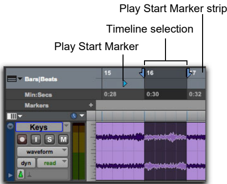
Dynamic Transport mode, Play Start Marker shown in expanded Main Timebase ruler
