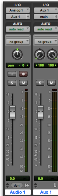
New Auxiliary Input track with audio track output automatically assigned to Bus 1–2
