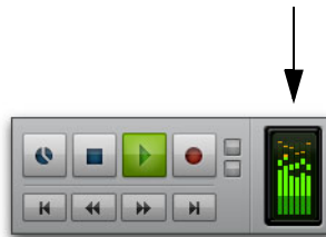
Output Meters channel order determined by the Output configuration in the I/O Setup
