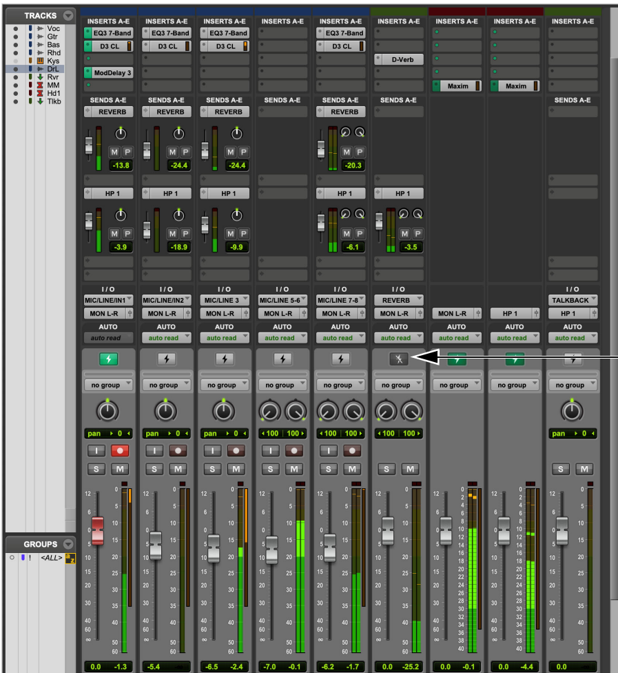
Figure 5. Session configured for recording vocals, but with Auxiliary Input track in DSP Mode Safe for Native reverb processing
