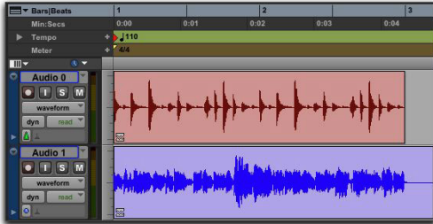
A multitrack clip group separated across sample-based and tick-based tracks after changing tempo
