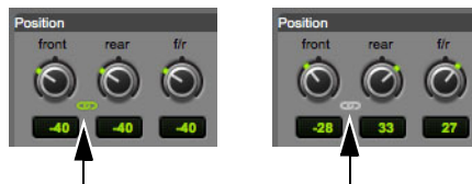
Front and Rear positions linked (left) versus Front and Rear positions unlinked (right)
