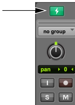
Track DSP Mode button enabled: in the Edit window (top) and in the Mix window (bottom)
