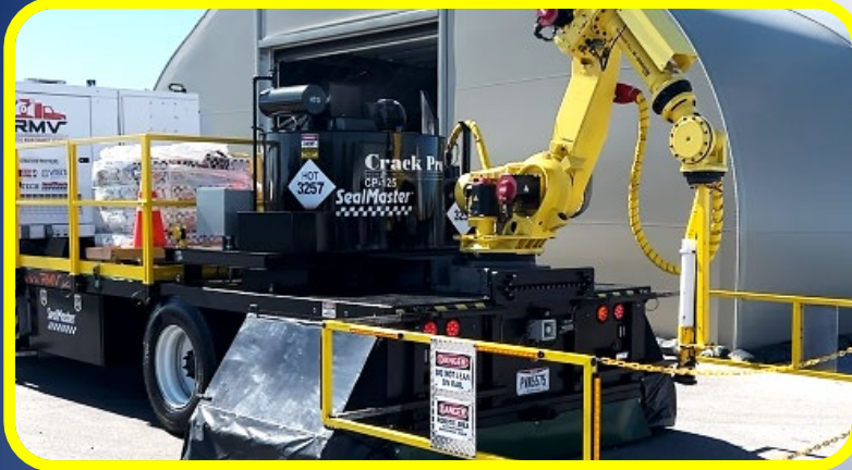
NecoPave Automatic asphalt fill and repair machine for use on existing roadways; increasing the efficiency of pavement repairs
