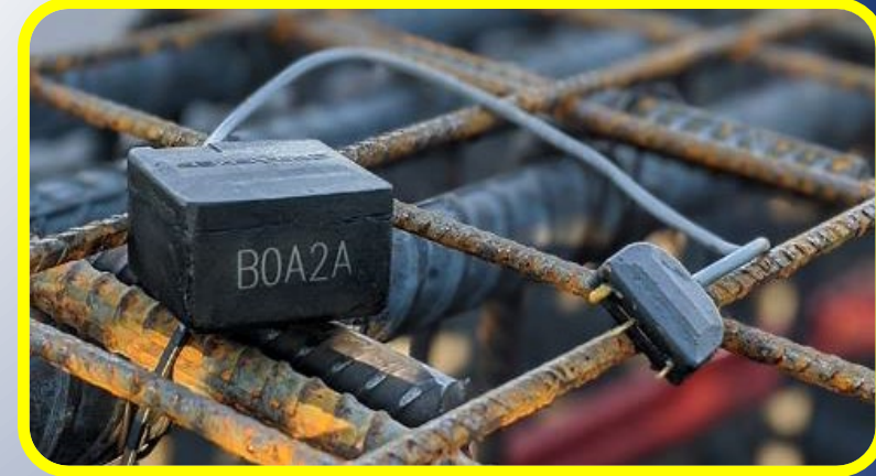
Sensytec Sensor that monitors temperature and electrical resistivity for assessment of concrete structural damage and soil contamination
